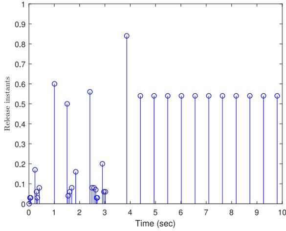
Fig. 6. Releasing sequence under the proposed adaptive METM.
