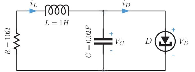
Fig. 3. Tunnel diode circuit.
